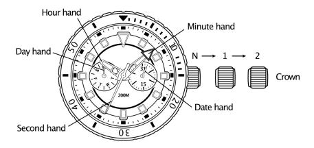
◆ Crown operation – You must unscrew the crown counterclockwise to release before pulling.
